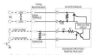
\* Control line is compatible with totem pole or tri-state output device.
